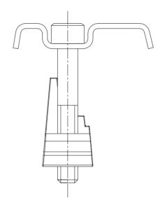
This block is a true representation of a BeamClamp Gratefix. It is designed to allow open floor grating to be connected to the supporting steelwork without any penetration of the steelwork and no access to the underside is required. Please refer to web site or technical literature for full details of its use. www.beamclamp.com/resources/beamclamp-configurator Kee Safety Ltd
